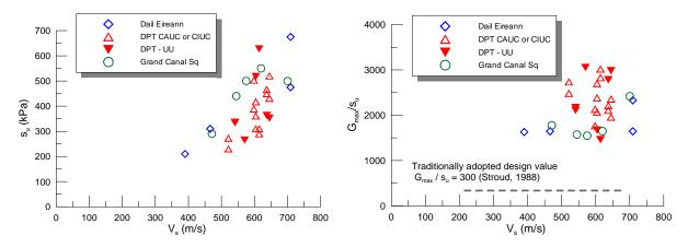
Figure 4: The variation of  $V_s$  with (a)  $s_u$  and (b) the design parameter  $G_{max}/s_u$
