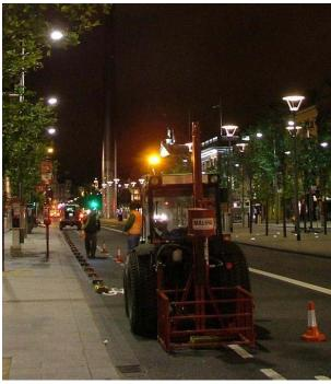
Figure 3: Acquisition of 2D roll-along MASW data in Dublin city centre.
