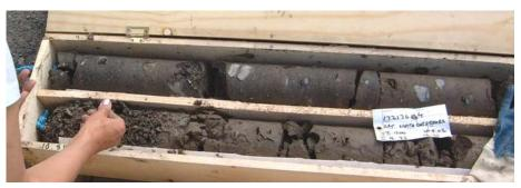
Figure 1: Geobore-S core of Dublin boulder clay showing distinct sand or silt lens within the largely clay matrix (Skipper et al., 2005)
