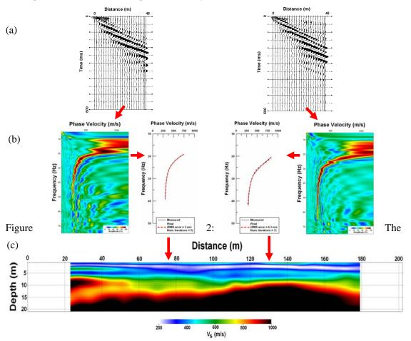
various stages involved in producing a 2D MASW profile, in this case from a Dublin city centre site, south of the river Liffey: (a) raw seismic data, (b) dispersion curve image and inversion and (c) 2D  $V_s$  image combining inverted 1D  $V_s$  profiles.
